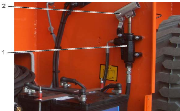
Hand pump for the extendable part of the platform
