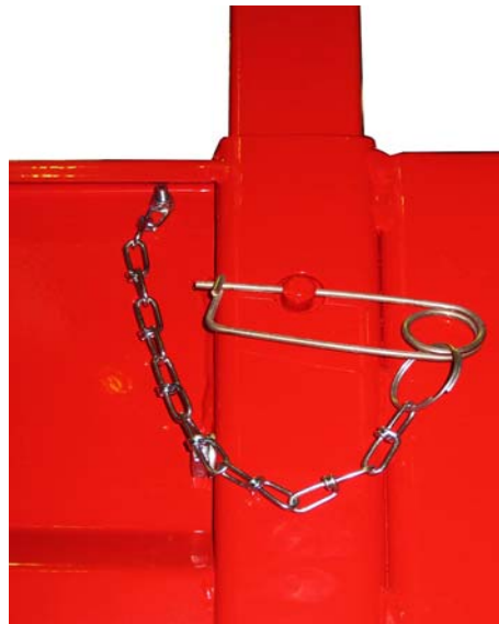
Closed scissor skirt lock on the platform
